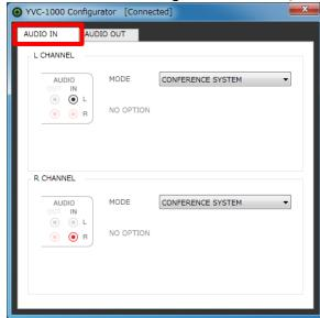
5. Set "PA MICROPHONE" in "MODE" of the terminal to which the XD-V35 receiver is connected.
