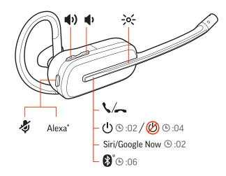
Power on or off Press the Call S button until you hear "power on" or "power off."
